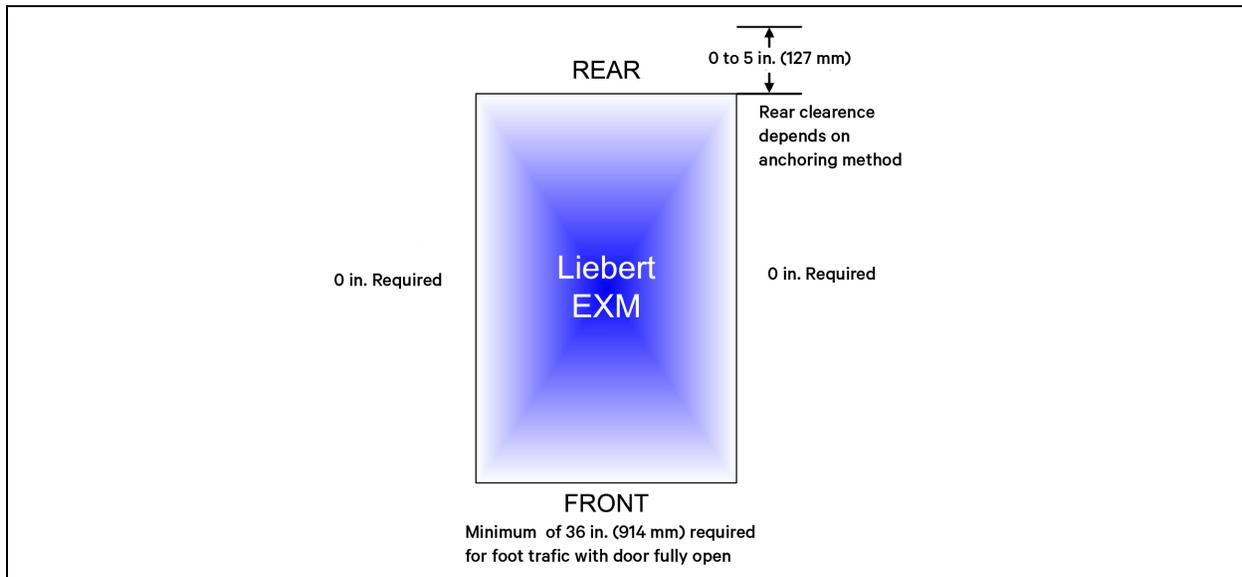
**NOTE: Minimum of 36 in. (914 mm) required for foot traffic with door fully open.**
