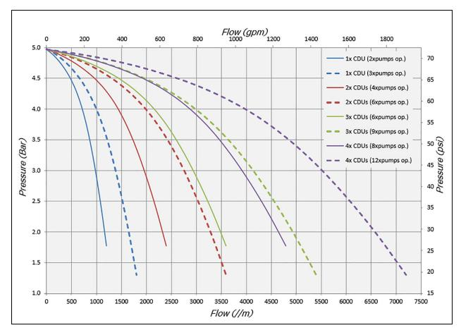
Figure 4.7 Flow/Pressure Graphs for Multiple Units (pumps) in Parallel
