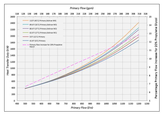
Figure 4.5 Primary Flow/Temperature Graph for 12.6°F (7°C) ATD
