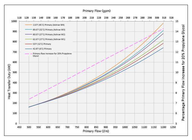
Figure 4.3 Primary Flow/Temperature Graph for 5.4°F (3°C) ATD
