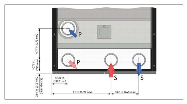
Figure 3.4 Rear Section Showing Primary and Secondary Pipe Connection Locations
