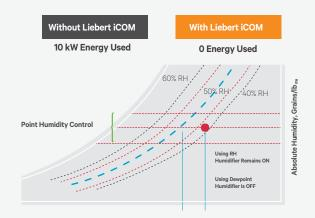
The dew point control routine operates humidification and dehumidification from dew point instead of relative humidity. This prevents activation of these components based on large temperature changes, thereby saving energy.
