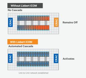
Automatic cascade and lead/lag routines activate and deactivate units based on room load to minimize hot spots and overheating.
