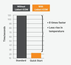
Recovery times from loss of power or transfer to generator power are reduced. Faster restart decreases temperature rise during these events.
