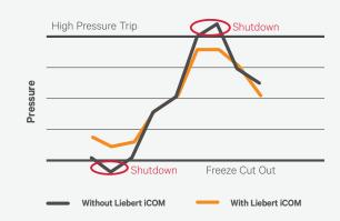
Self-healing routines prevent DX refrigerant freeze. As refrigerant pressure approaches thresholds, the controls lower fan speed and compressor capacity so cooling is not disabled due to a low-pressure cut out. At the other end of the spectrum, the controls adjust the compressor down and raise fan speed so cooling is not disabled due to a high pressure condition.
