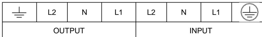
If an optional POD with attached input cord and output receptacles are used, connect the input to a L14-30 receptacle and connect the user supplied equipment to the output receptacles.
