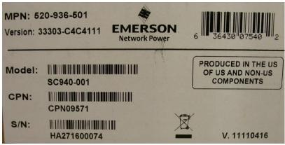
On your switch unit, locate the white Emerson Network Power sticker. On the right-hand side of the label, under the Emerson logo, the unit serial number (S/N) will be indicated with a combination of letters and/or numbers listed below a bar code. For example, the serial number is HA27160074 as indicated in the following graphic.
