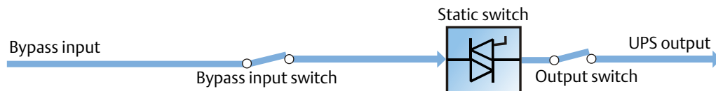
Figure 1-5 Bypass operating mode line diagram
