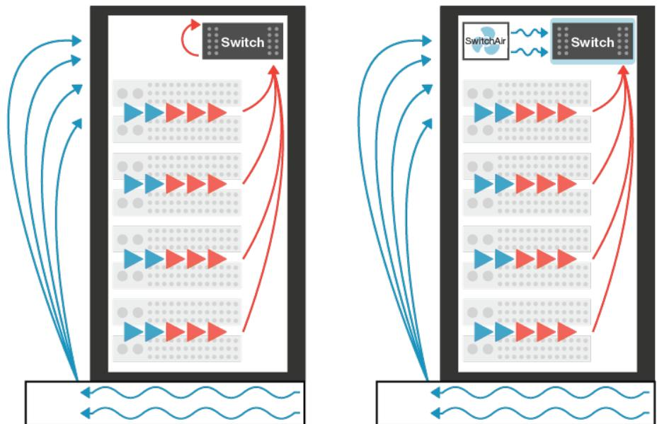
*Network switches mounted at the top and rear of the rack are susceptible to heated air from the servers. This hot air is recirculated, putting stress on the device.*
