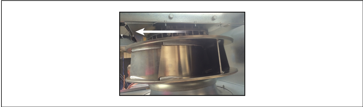
Figure 9.10 Slide the Fan Assembly Out of the Front of the Unit
