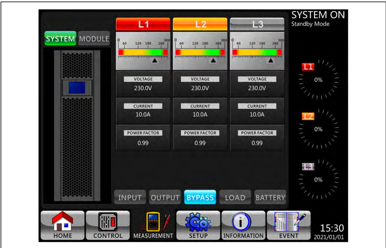
Figure 4.9 System Measurement Screen-Bypass
