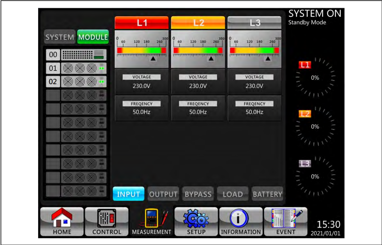
Figure 4.12 Module Measurement Screen-Input
