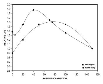
**Figure 1 – Relative life of vented lead-acid batteries as a function of positive plate polarization** Source: Presentation by Sudhan Misra, C&D Technologies at the Critical & Backup Power conference, Boston, MA, November 2003
