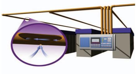
Figure 4 – Air-Sampling Smoke Detector
