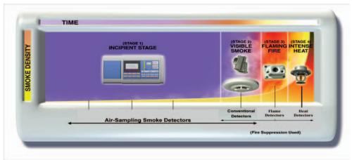
Figure 1 – Typical Fire Growth Curve and Detection Types
