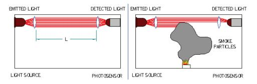
Figure 3 – Projected Beam Smoke Detector
