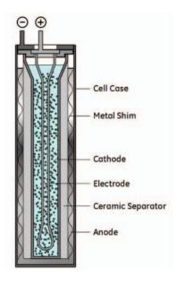
Figure 1 – Cell Schematic
