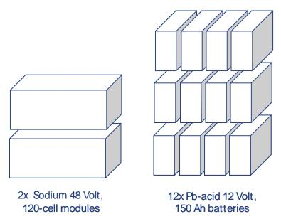
Figure 2 - Telecom Cabinet Battery Comparison
