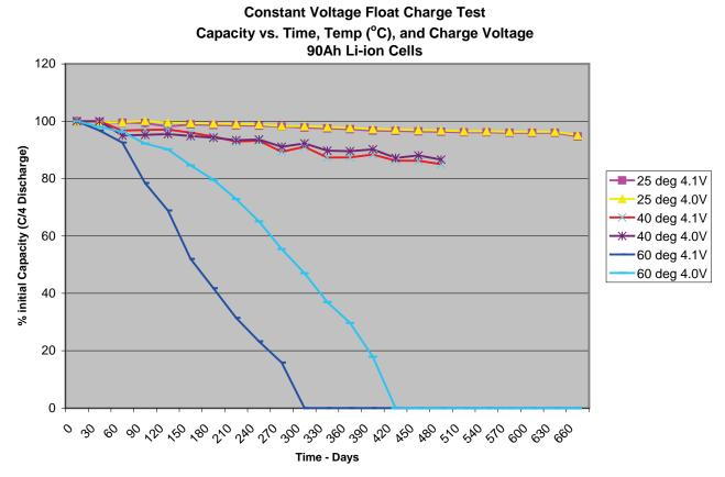
Figure 4. Lithium-Ion Cell Temperature and Voltage Effects
