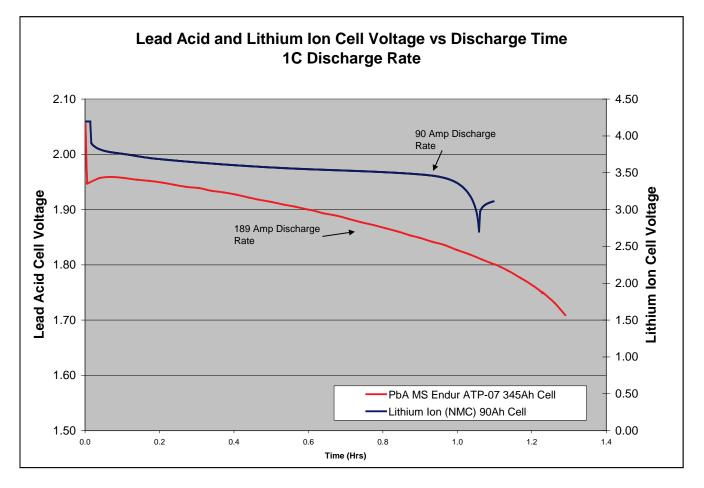
Figure 5. Discharge Curve Comparison: Lead Acid versus Lithium Ion
