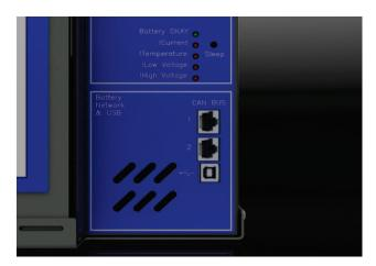
**Figure 7. Example of External Communication Connections**
