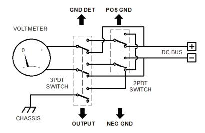
**Ground Detection Voltmeter**
