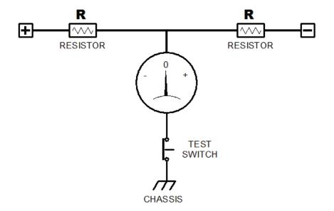
**Ground Detection Ammeter**
