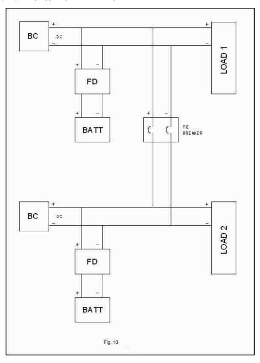
Two battery chargers and two batteries with tie breaker
