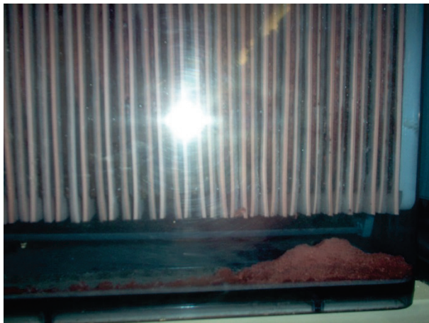
Figure 18. Shed active material.
