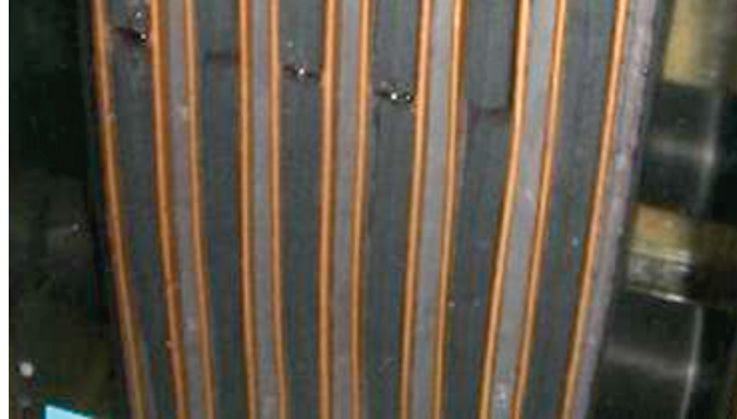
Figure 12. Cracked positive plates.
