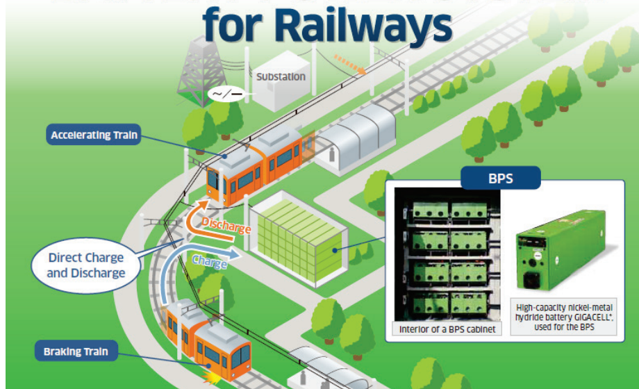
Figure 8. Illustration of a wayside railroad BPS installation. (Courtesy Kawasaki Heavy Industries)
