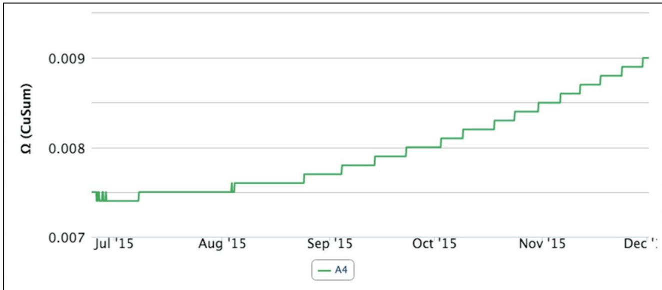
**Figure 3. Change in DC resistance with time for a VRLA battery in a 48V string.
