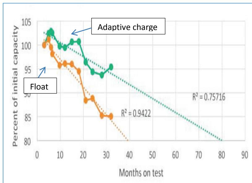
**Figure 1: Life predictions of batteries on continuous float and operated by the adaptive charge management system. Test temperature = 40°C.**
