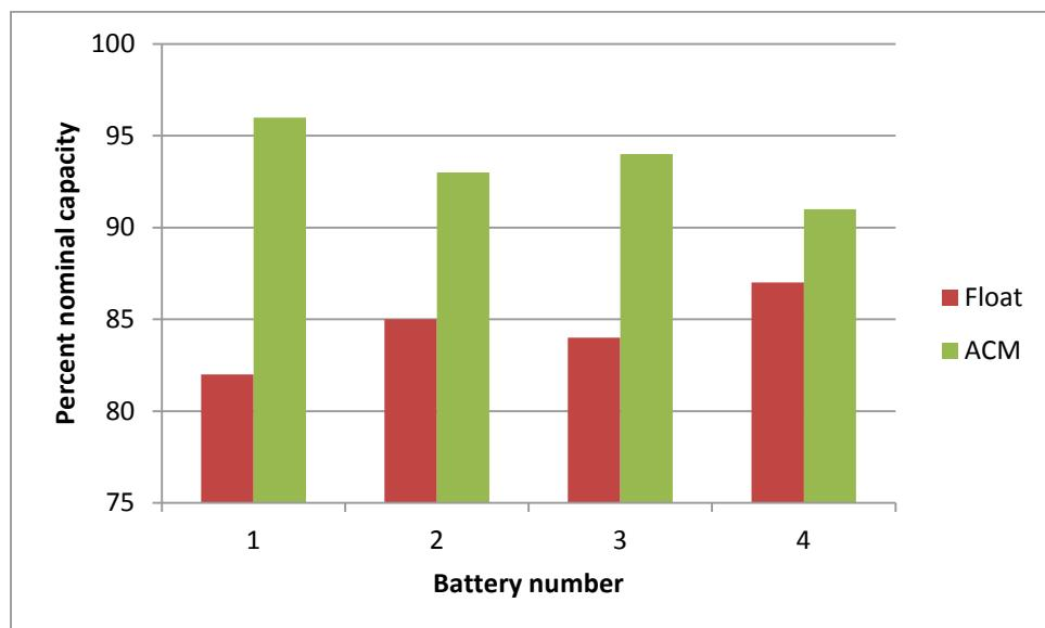
**Figure 5. Comparison of capacities of batteries on float to batteries on adaptive charge after 21 months.**
