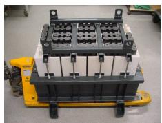
This performance is reached in both vertical as well as in horizontal orientation of plates, as it is shown in the figures. Here UPS batteries sets are shown during homologation tests concerning earthquake and shock impact. All sets are based on 2V / 1000 Ah cells in VRLA / AGM technology.
