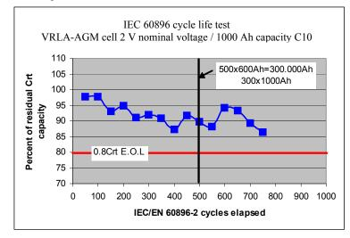
After 50 of such cycles and without any equalization or boost charge, determine the residual capacity of the units with a  $C_{10}$  discharge to 1.80Vpc, the results are shown in the diagram.
