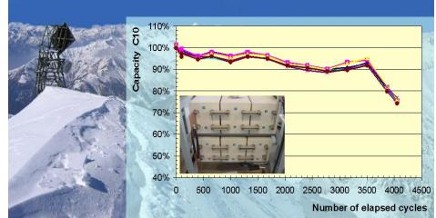
Solar cycle service : 6 month/y at 17-25°C, 6 month/y at 22°C-35°C daily cycle : discharge= 24% DOD / 12 h, recharge= 0.6\*I10 / 12h discharge with 100A to 1.82Vpc, in % of the rated capacity
