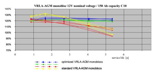
The need for improving service life time is especially for elevated ambient temperature conditions. Therefore a test result is presented for float voltage charging test with periodically capacity (c3) testing on VRLA-AGM monoblocs with 2V nominal voltage / 150 Ah capacity.
