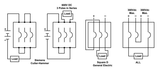
If a grounded battery of over 250VDC is used then a UL listed bolted pressure switch may be used.
