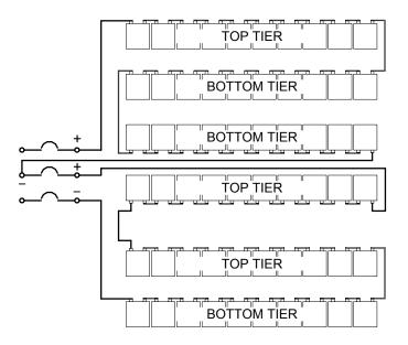
Sectionalizing a Lower voltage Battery on Three Two Tier Racks by Using a Three Pole Device
