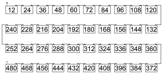
If during servicing we interrupt the connection between jars twenty and twenty-one then the voltage is halved.
