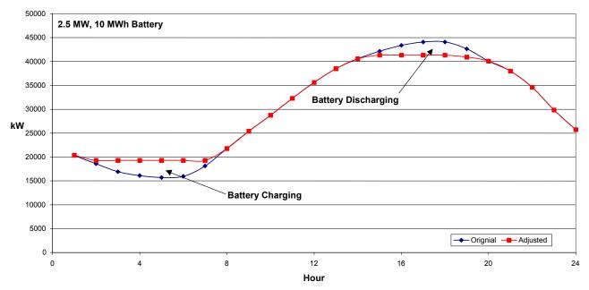
Figure 1. Sample Peak Shaving Operation for June 30, 1999.
