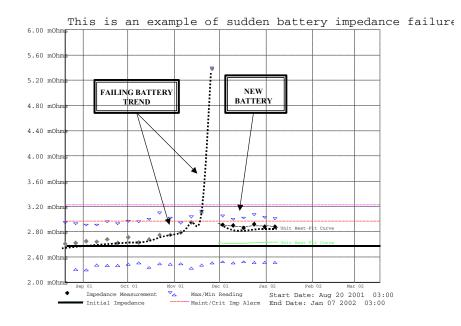
If this battery string was inspected once a quarter, the odds of finding and correcting this failing jar are not good.
