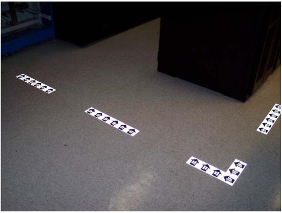
Figure 5. Equipment aisles identified with color coded reflective decals for zoned emergency power disconnect
