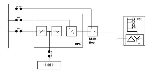
Figure 2. Block diagram of a traditional double-conversion non redundant ac UPS system
