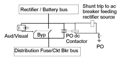
Figure 8. A zoned power disconnect arrangement with a bypass feature for system tests
