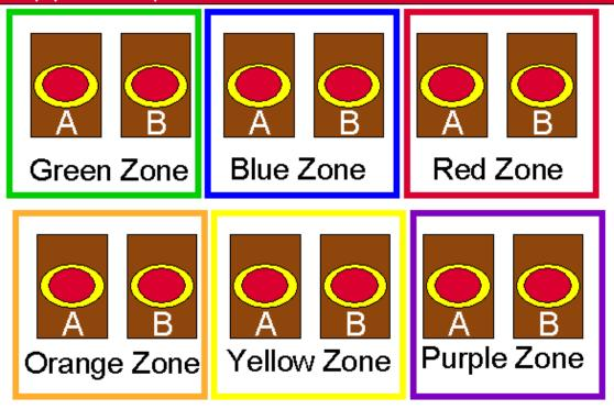
Figure 7. A zoned power disconnect arrangement for facilities with distributed dc (6 zones are shown in this example).
