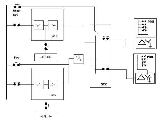
Figure 3. Block diagram of a traditional double-conversion redundant ac UPS system
