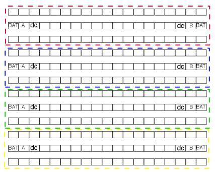
Figure 6. Equipment aisles identified with color coded reflective decals for zoned emergency power disconnect
