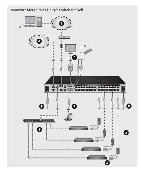
cable to the PDU1 port on the switch. Connect the other end to the PDU. Connect the power cords from the target servers to the PDU. Connect the PDU to a power source. Repeat this procedure for the PDU2 port to connect a second PDU, if desired.
