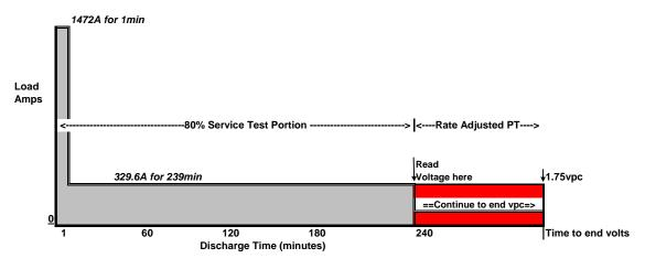
Figure 1. 4-hour Test Profile to 1.75 VPC
