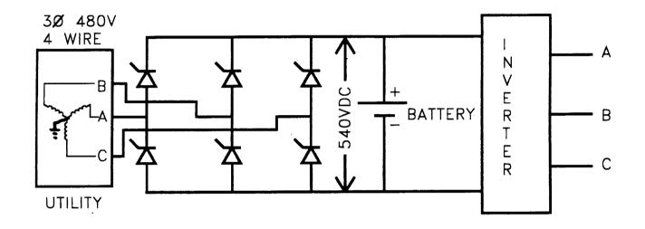
Figure 2 UPS Schematic
