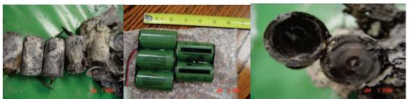
Photos taken by PHMSA inspectors as part of their investigation into a reported battery fire in a small parcel air carrier facility.
