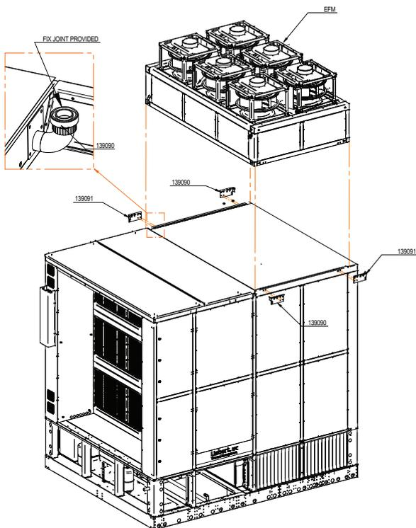
2. Put the gasket on the heat exchanger module, fix the four brackets on heat exchanger module.
