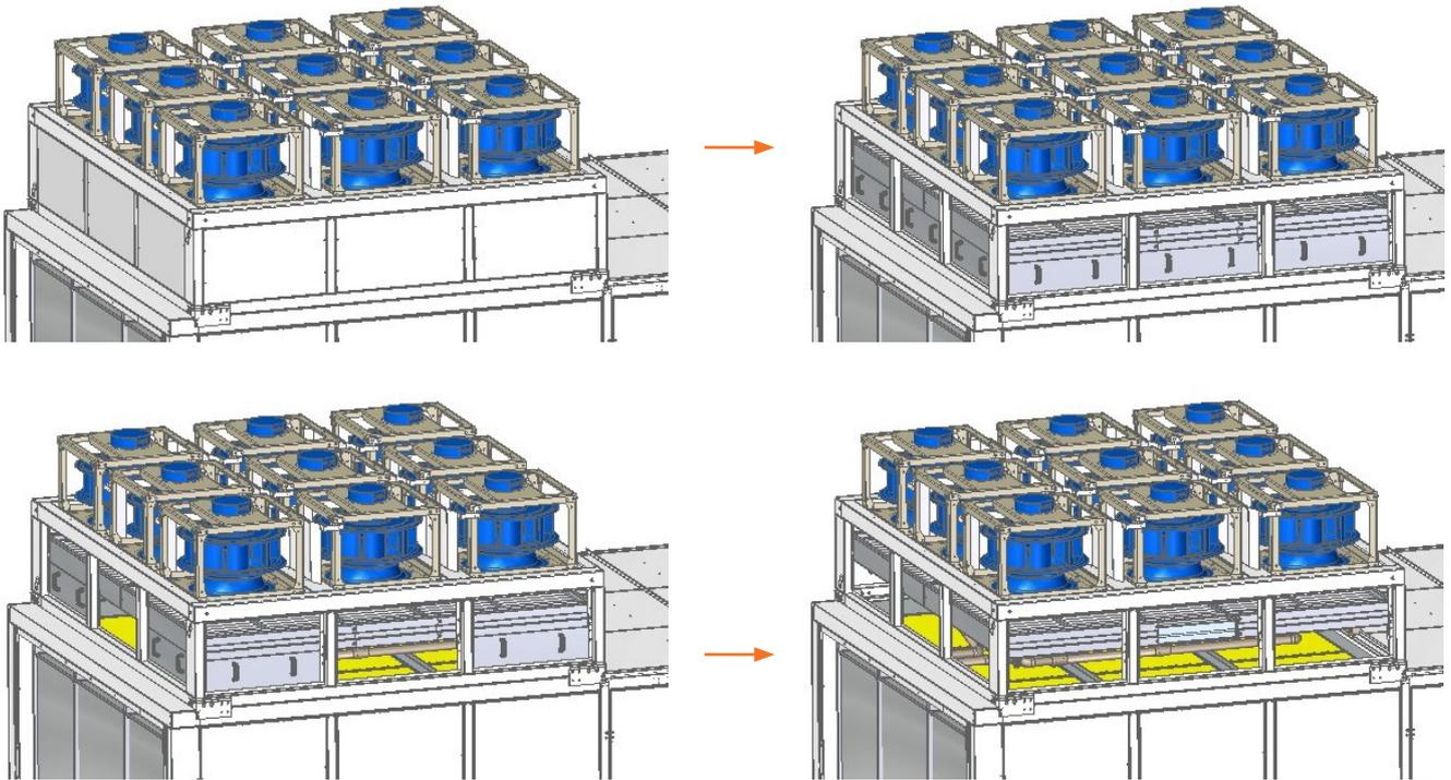
With Low Ambient Kit option, rotate the damper upwards to access to external air filters.
