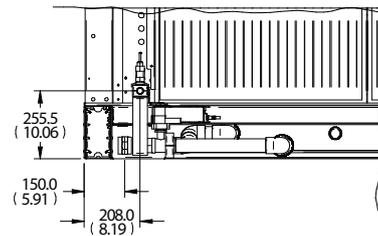
The water and drain connections of the Liebert® EFC440 unit are presented in the picture below.
