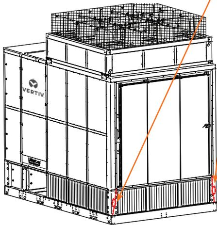
**Condensate drain:** the unit is supplied with 2 traps placed on condensate drain panel bottom. The condensate is discharged on unit basin. Fill in the drain trap with water before unit start-up.
