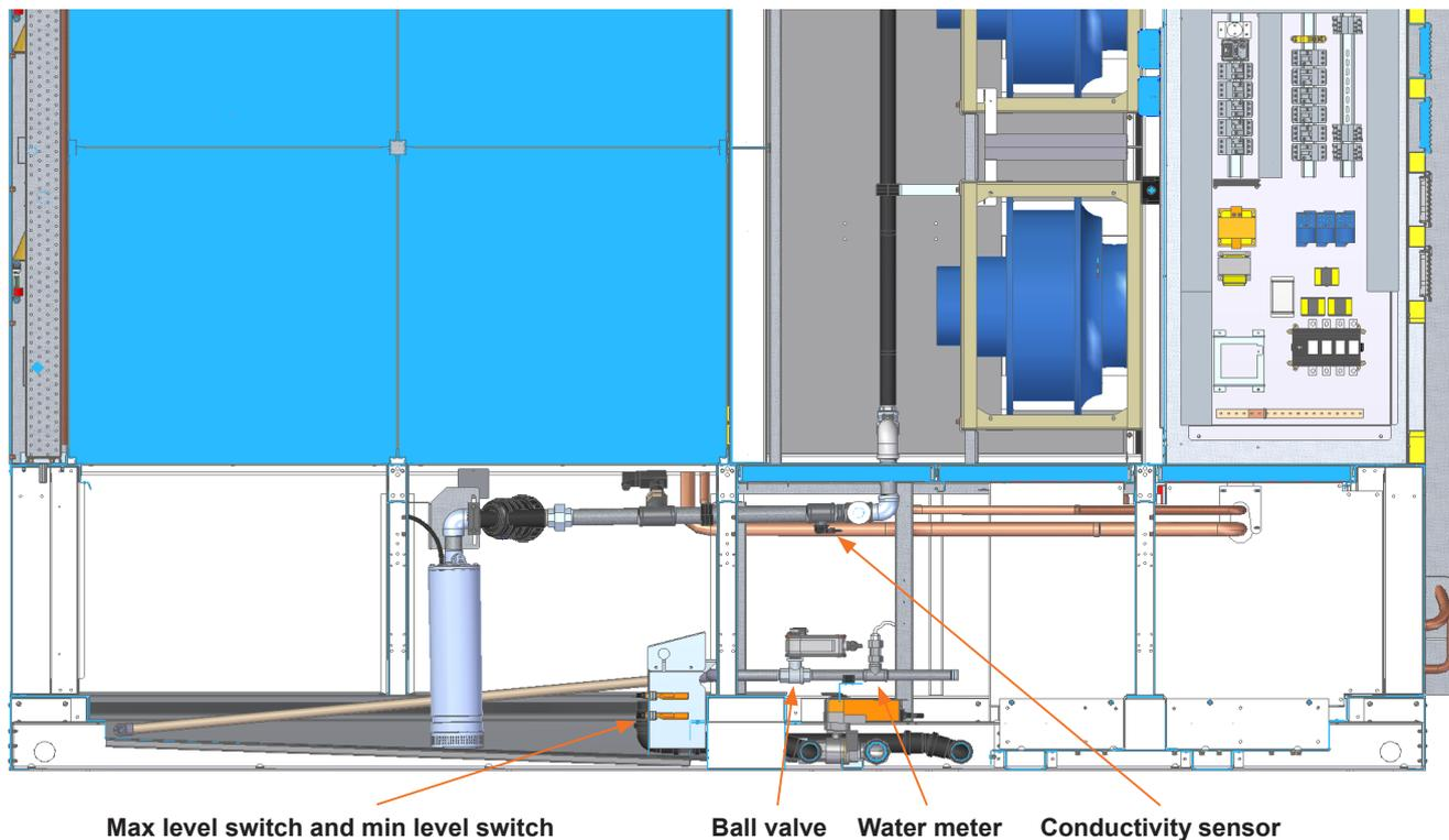
Max level switch and min level switch
