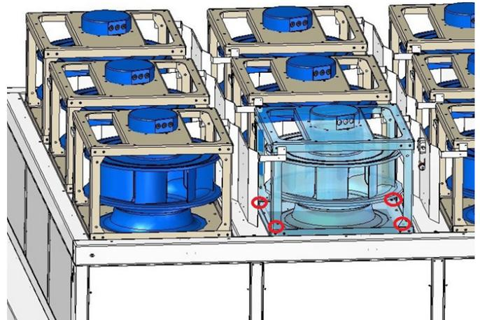
2. Remove the fan assembly from the unit.
