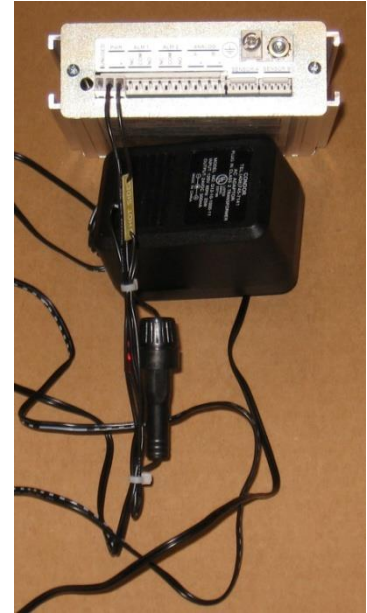
Figure 91. Multitel's FCCP with Power Source And Inline Fuseholder
