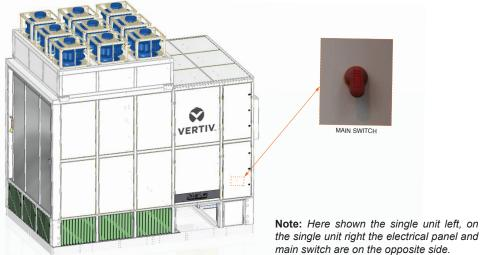
Unscrew the door and open it to access the main switch.
