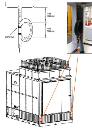
**Condensate drain:** the unit is supplied with 2 traps placed on condensate drain panel bottom. The condensate is discharged on unit basin. Fill in the drain trap with water before unit start-up.
