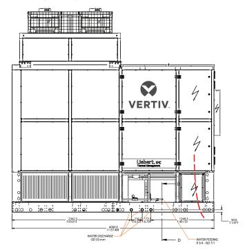
The water and drain connection of the **Liebert**<sup>®</sup> **EFC220** unit are presented in the picture below.
