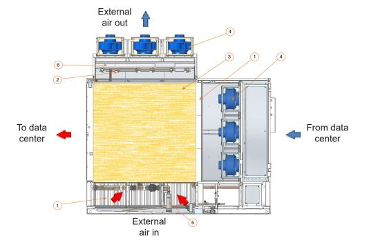
In climates featuring high levels of humidity the unit requires the integration of a **Direct Expansion** (**DX**) System or the installation of a **Chilled Water** (**CW**) Coil.
