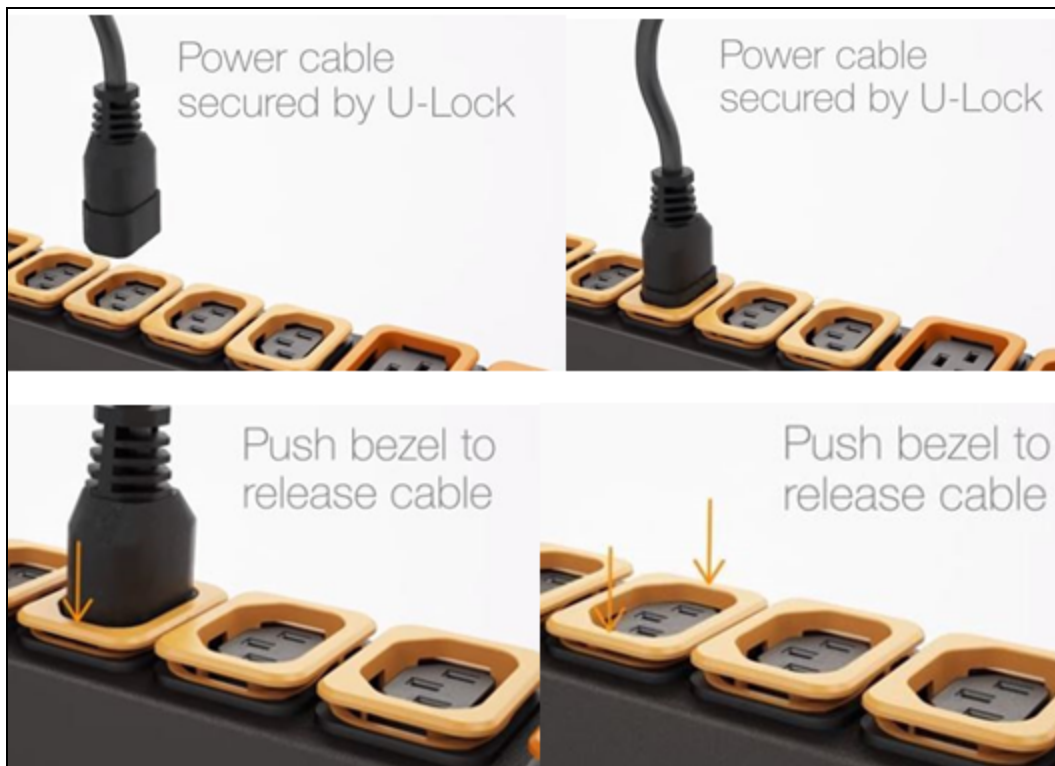
Figure 2.15 U-Lock Cord Retention Operation
